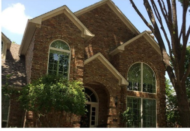
This house design has a complex massing where the gable elements are competing for importance. The window openings are too large and out of proportion for the façade. This home has a complex massing where the gable elements are competing for importance.
